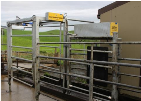
This installation includes an auto drafter. An EID panel reader and antenna have been installed at the end of platform.
